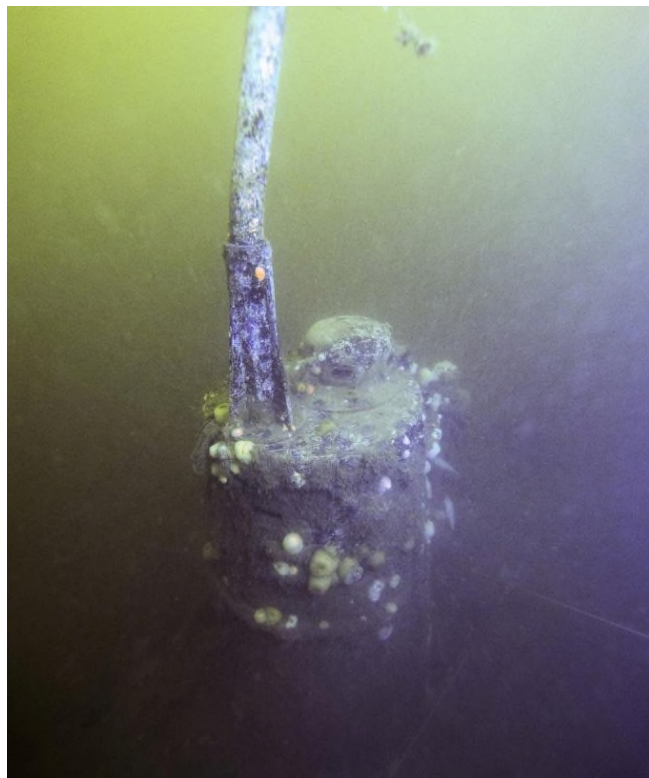
Figure 51: Conning tower top and periscope from the port side looking aft. The bend in the periscope can be seen just above the supporting collar
