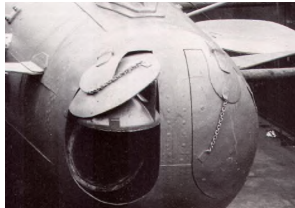
Figure 35: The same design of torpedo tube, bow cap, shutter and inspection panel on submarine C1
