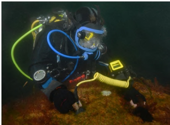
Figure 62: Testing the Cygnus DIVE gauge underwater on a wreck off Plymouth
