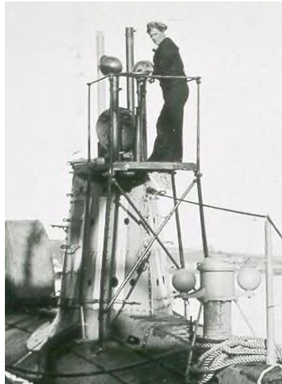
Figure 52: The flying bridge on A7 from aft. The two ventilator tubes and cowls can be seen aft of the open main hatch
