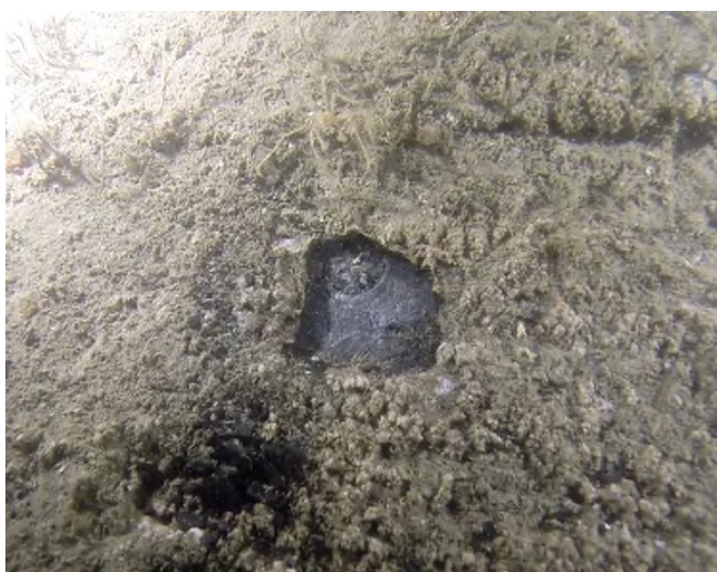
Figure 61: A small area of concretion removed to show the bright but uneven and pitted metal underneath
